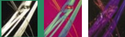
Chrysotile Asbestos - PLM
