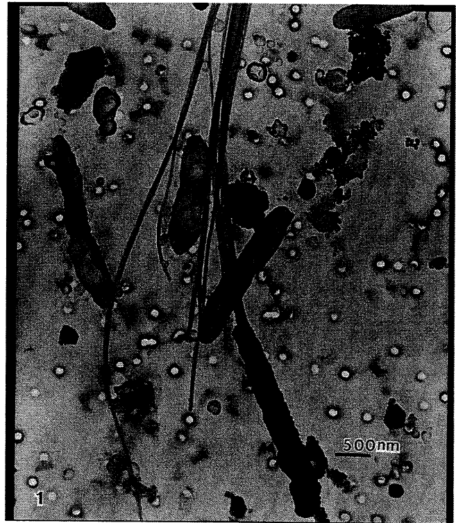
FIG. 1. The ferruginous body in this micrograph is formed on a bundle of chrysotile fibrils. Original magnification 20,000 \times .
